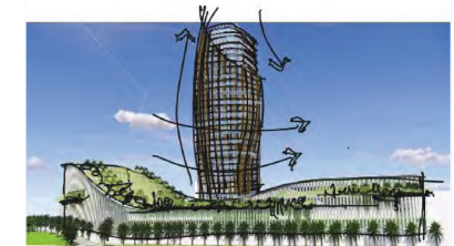
Peeling away the mullions to reveal upper level apartments with terraces enjoying a northern view
